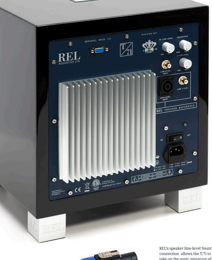
REL's speaker line-level Neutrik connection allows the T/7i to take on the sonic signature of the amplifier it's connected to. A line level connection is also offered, but this is a simple, elegant and cost effective solution.
