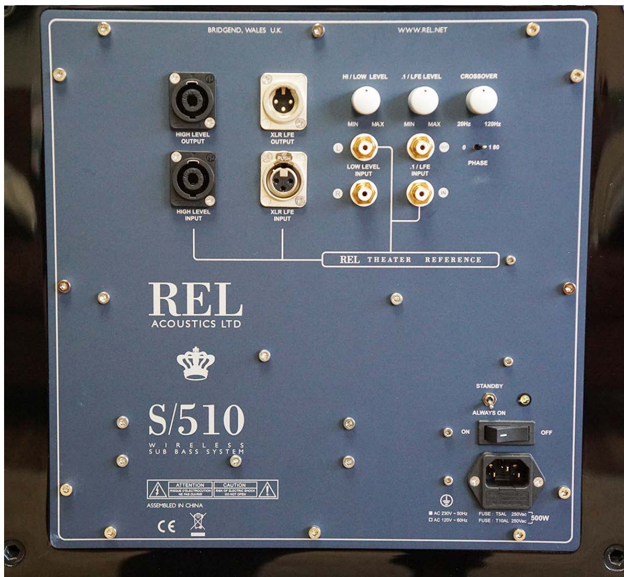
The S/510's rear panel is clearly laid out, with XLR (balanced), RCA and Speakon connectors plus volume and crossover trim pots
